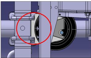
Fasten the air spring to the Upper Bracket using the 3/8" hex head bolt.
