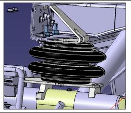
Make sure that the end of the Lower Bracket fits between the U-bolts on the leaf springs **making** it impossible to rotate the bracket.
