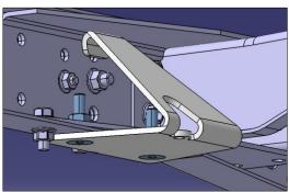
For vehicles with taller frame, fit chassis extension piece using M8 x 20 Hex Head Bolt. (Left hand side Shown)
