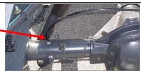
Replace with the new replacement "De-Breather Tube" that is supplied with the kit.
